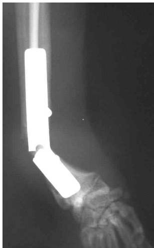
Fig. 8: DCP failure after multiple plate bending through plate hole
